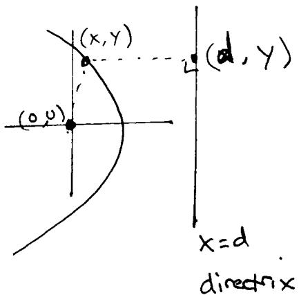
$$\frac{\text{origin-to-(x,y) distance}}{\text{directrix-to-(x,y) distance}} = e = \text{eccentricity}$$
