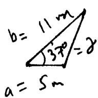
$$\text{Area} = \frac{1}{2} ab \sin \gamma = \frac{1}{2} (5\text{m})(11\text{m}) \sin 37^\circ \\ = 16.54 \text{ m}^2$$
